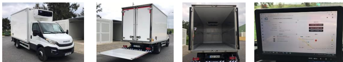
Picture 5. The refrigerator track for the food waste collection system from hotels
