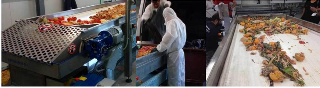
Picture 7. During hand sorting on the conveyor belt in the pretreatment unit
