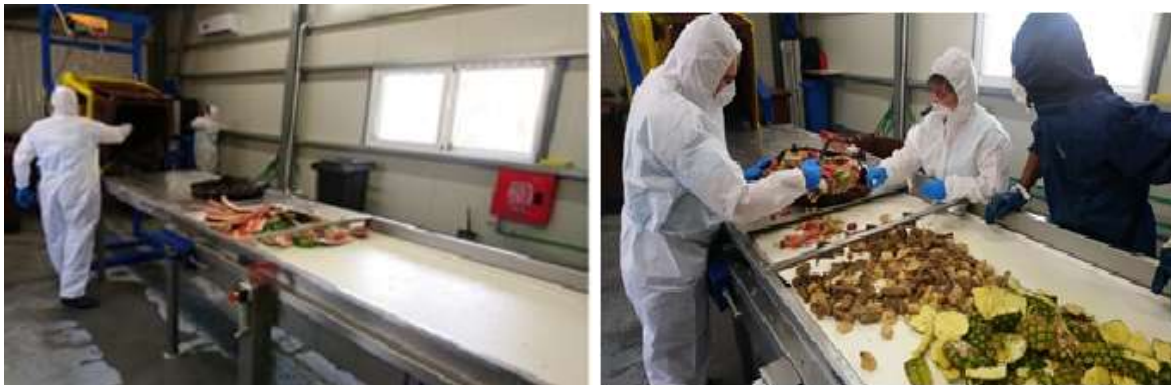
Figure 5: Import and hand-sorting of the source-separated food waste in the pilot scale facility
