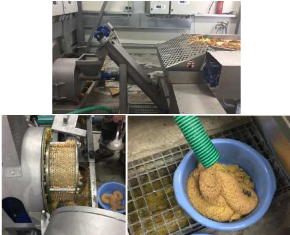
Figure 7: The pulp after the shredding process
