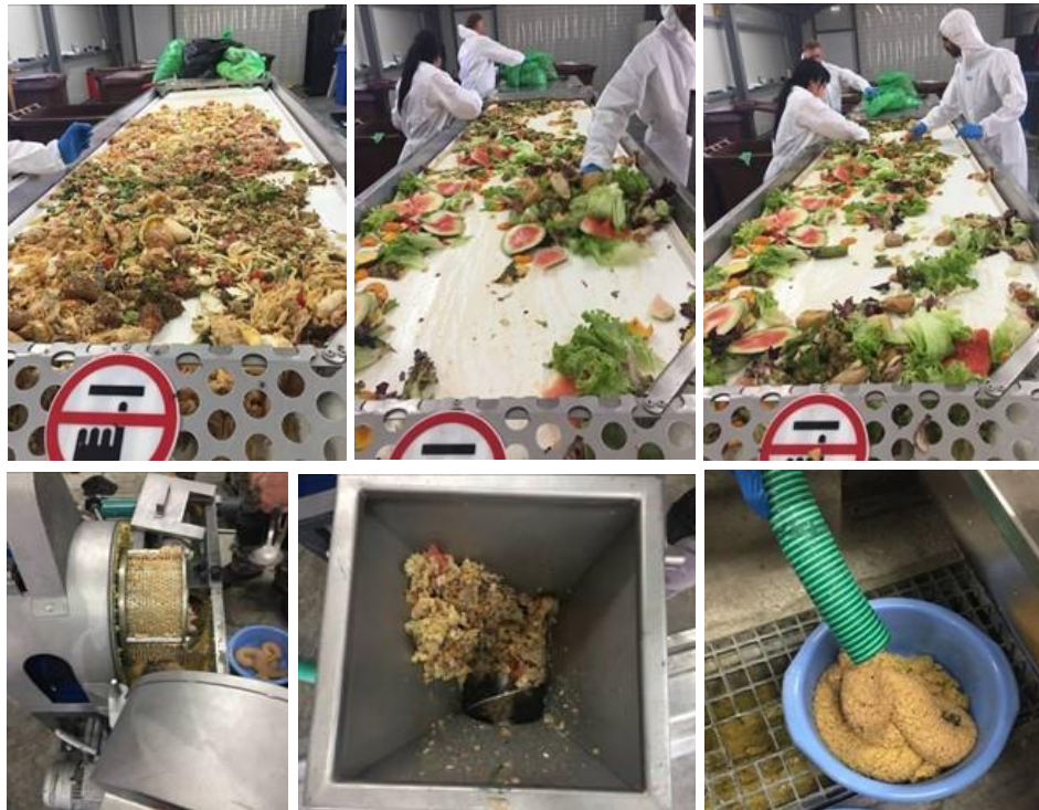
Picture 10. During the start-up of the second operational period of the F4F pilot unit. The food wastes after shredding and pulverising
