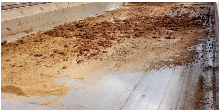
Picture 11. The final product after solar drying in the F4F pilot unit sent to partners
