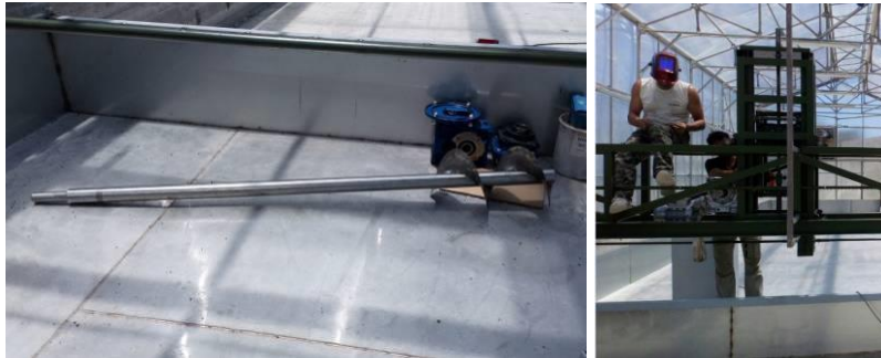
Picture 7. During transportation and installation of the vertical turner into the pilot unit
