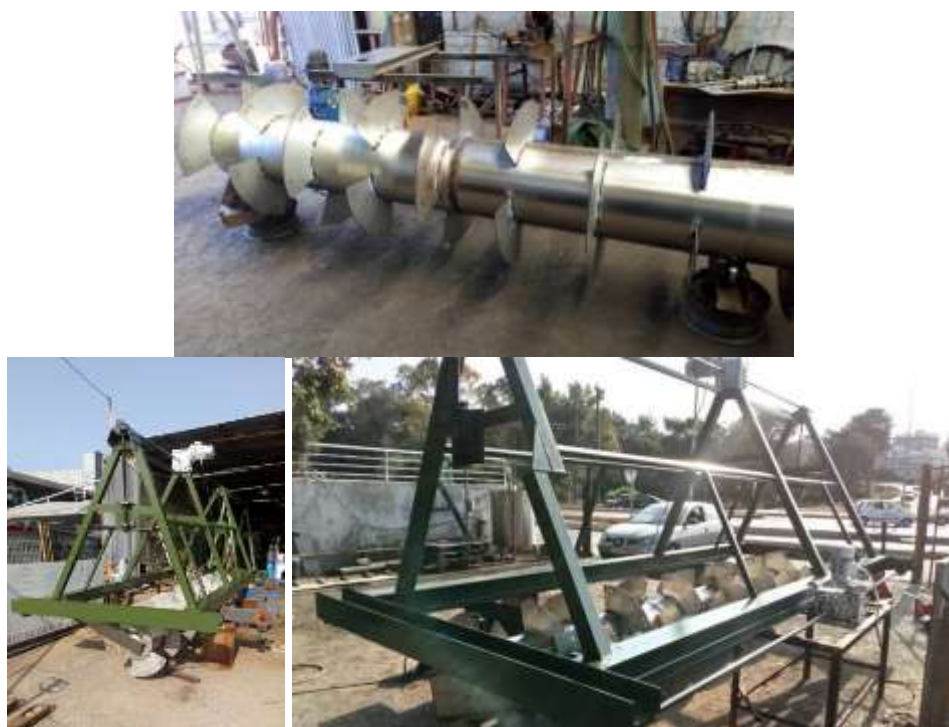
Picture 17. During the construction of the inox horizontal turner
